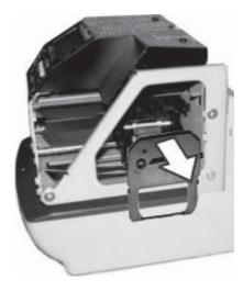
Turn the knob of the new cartridge in direction of the arrow (clockwise) to tighten the ribbon.
